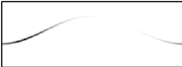
Figure 4: Sinogram. This is a standard sampling of the exponential Radon transform of a relative smooth pike. We present on this image the data. The horizontal axis is f ; the vertical axis is s .
