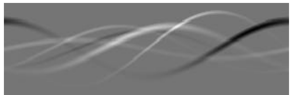
Figure 7: Sinogram. This is a standard sampling of the exponential Radon transform of a set of cold and hot areas in a constant active region. We present on this image the data. The horizontal axis is f ; the vertical axis is s .
