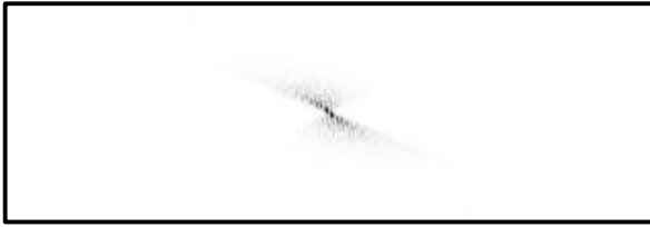
Figure 8: Modulus of the Fourier transform of the exponential Radon transform (see the data presented in Figure 7). We can recognize the bow tie shape indicating that interlaced sampling can be applied.
