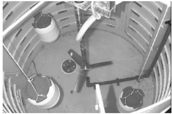
Figure 3. Photographic view of the 2.7 m 3 mixing tank filled with water together with three plastic bottles. The dimensions of the plastic bottles are 19 cm diameter and 27 cm high.
