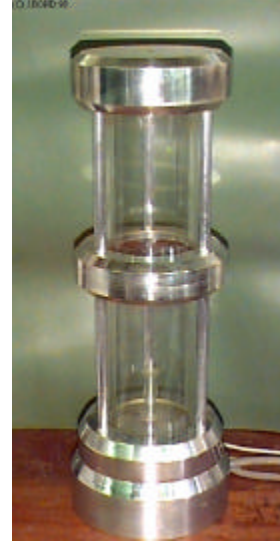
Figure 6 Bubble column with 16-electrode single plane sensor in centre of vessel
