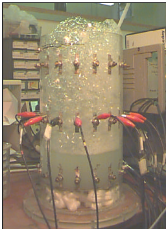
Figure 3: Experimental ERT foam column
