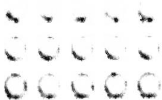
Figure 3: Tomographic images of a mixing process following a step change in solids concentration.
